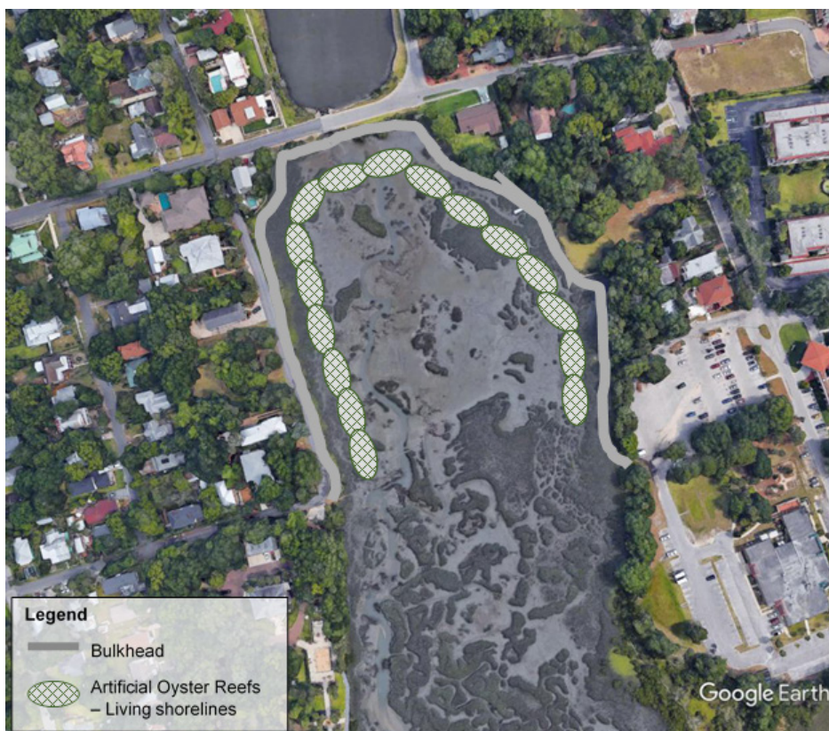
Figure 9. Location of bulkhead and the proposed location of artificial oyster reefs, at a regional scale.
